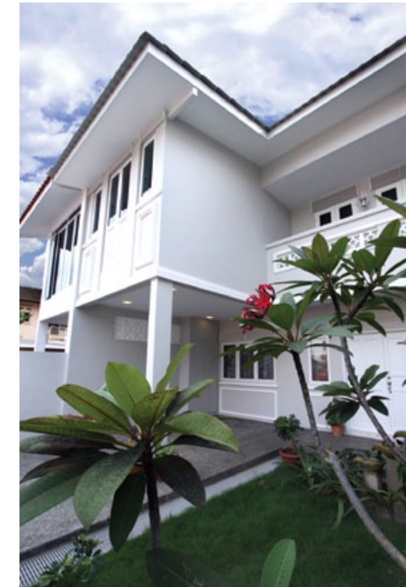
ABOVE: The use of double-shutter doors in the upper floors allows for air to flow through the rooms while maintaining the privacy of the room. The grey and white hues give a cool aura while minimalist detailing enhances the contemporary look.
